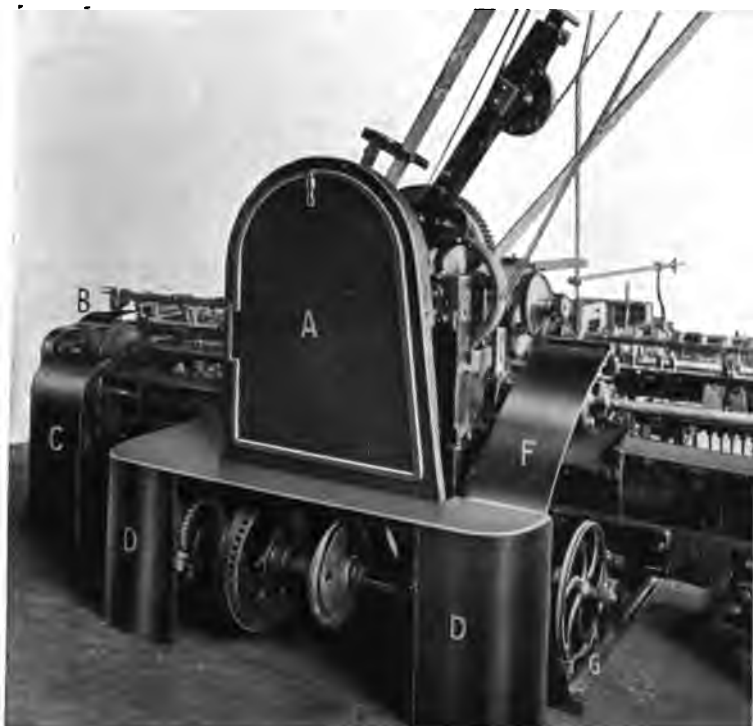
Fig. 1. Back view of Mule Head with Guards for Gears, Shafting, Pulleys, etc.
